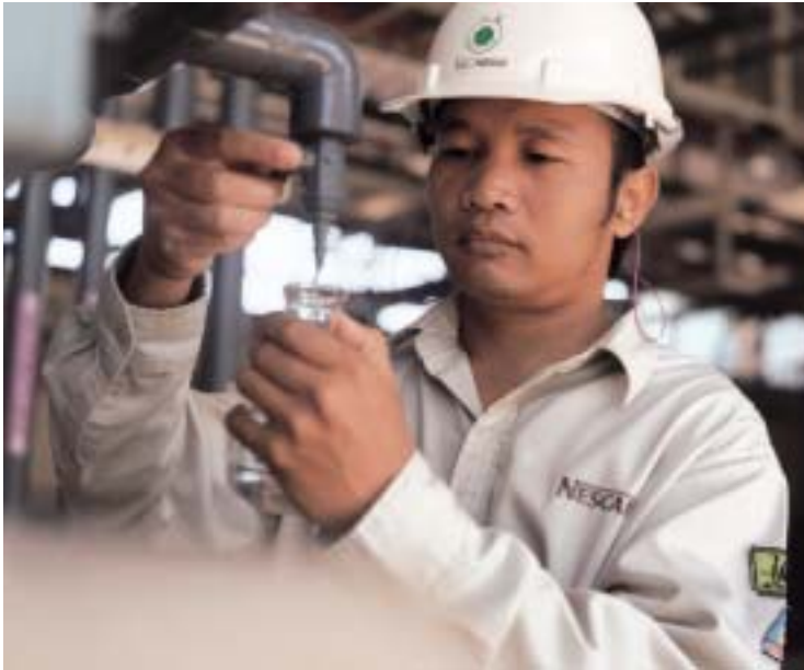
Left: Khun Taleungkiet at the Chachoengsao coffee factory in Thailand, testing the quality of water that has been treated for re-use. It is our first “zero water discharge” factory that recycles almost all water, either in cooling towers or for irrigation of an adjacent coffee nursery
