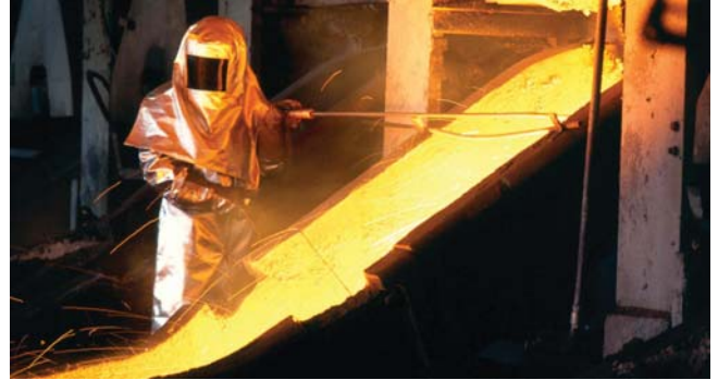
Titanium slag being tapped from a Rio Tinto smelter furnace using an oxygen lance
