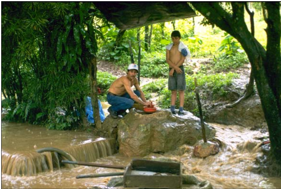
Placing the finely ground ore into a container to mix it with mercury and water.
