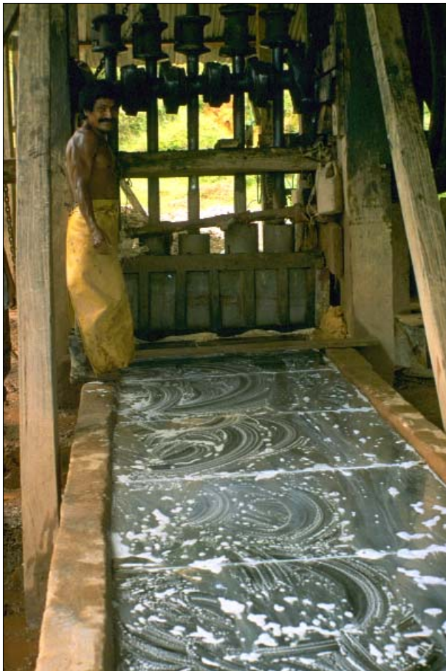
Ore that is finely ground is washed over this mercury-coated trough where a gold-mercury amalgam scum accumulates on the surface.
