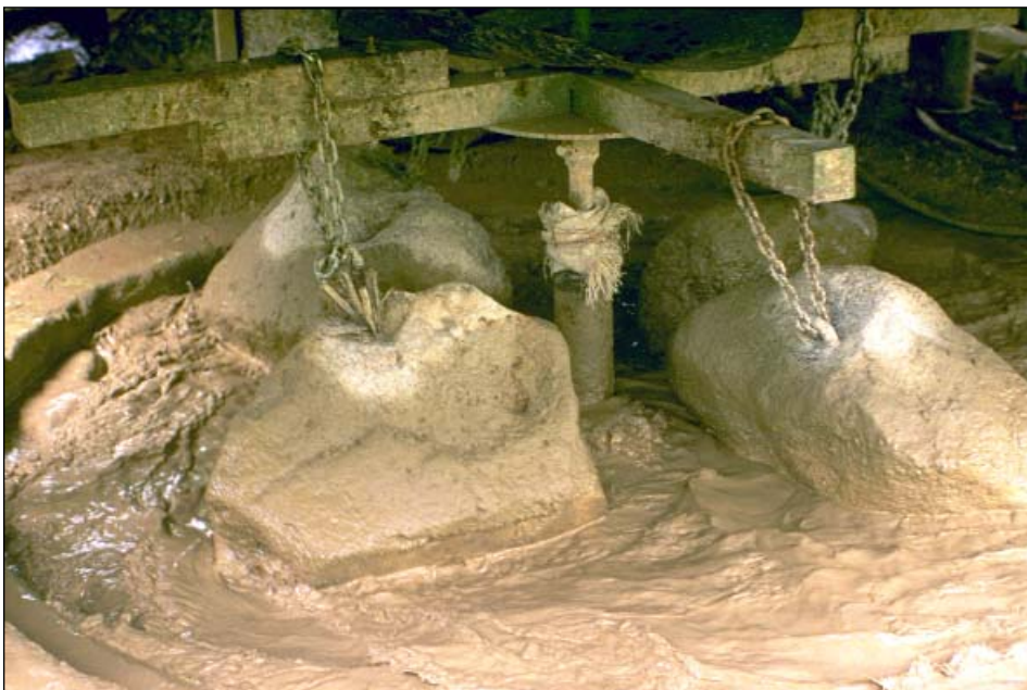
A traditional ore-processing "rastra", grinding high-grade ore.
