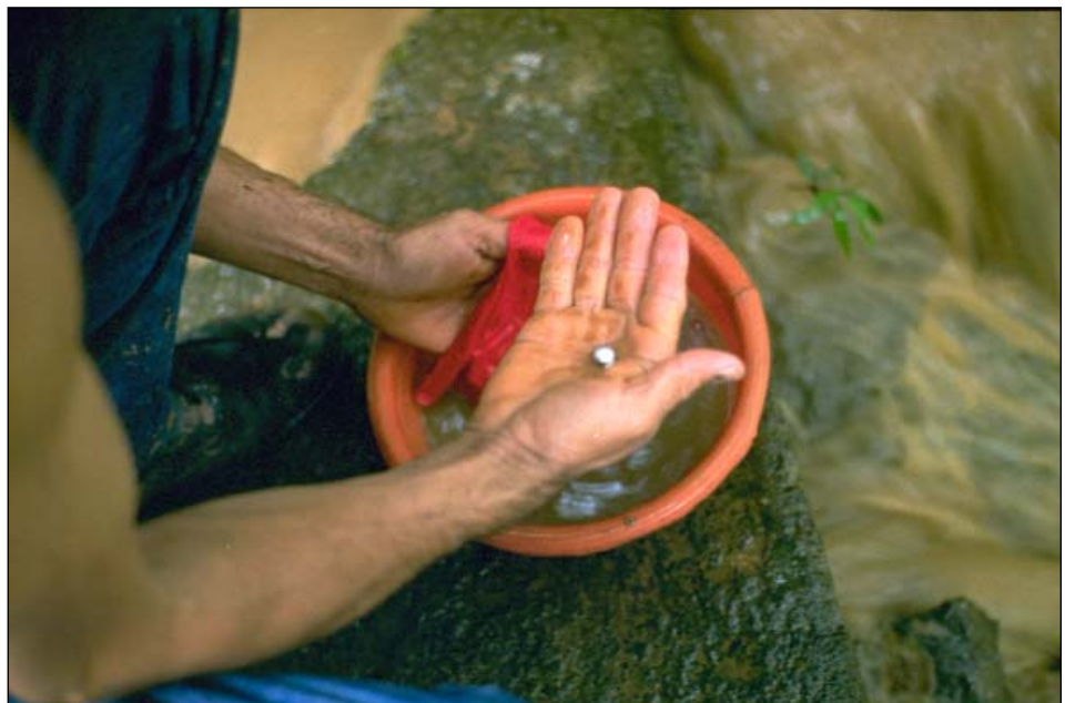
Amalgam of mercury with gold. One ounce of mercury was used to extract this ball containing 20 grams of gold.
