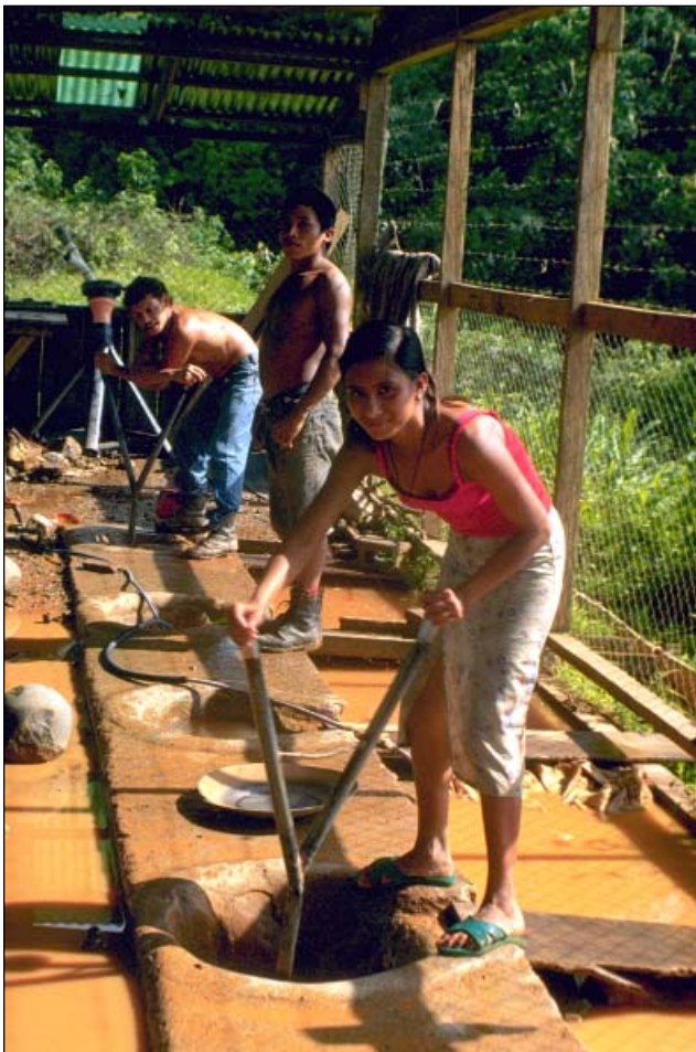
Manual ore-processing using "molinetes" for high-grade ore.
