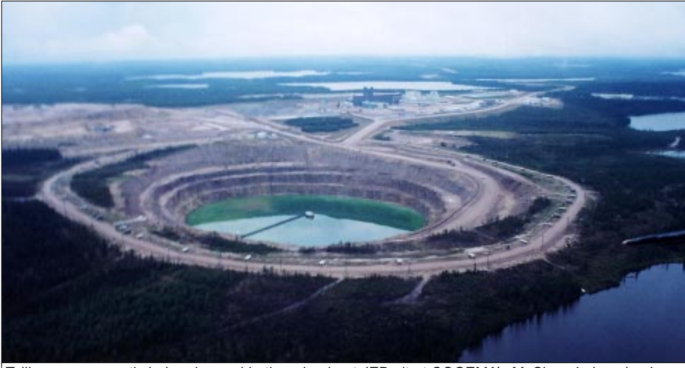
Tailings are currently being dumped in the mined-out JEB pit at COGEMA's McClellan Lake mine in northern Saskatchewan. R. Tsannie photo.
