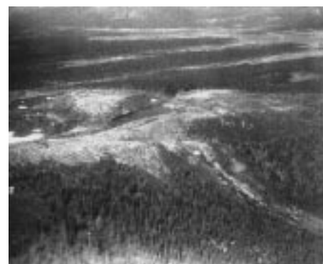
Aerial photo of the rust coloured outcrop that led to the discovery of the Voisey’s Bay nickel deposit.
